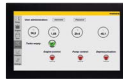
TX7xx HMI with PLC
