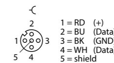
RFID channels (C0...C3) – Connectors .../S2503
